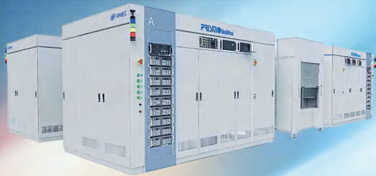
用于高性能Mini LED外延片量产的MOCVD设备 MOCVD solution for Mini LED mass production
